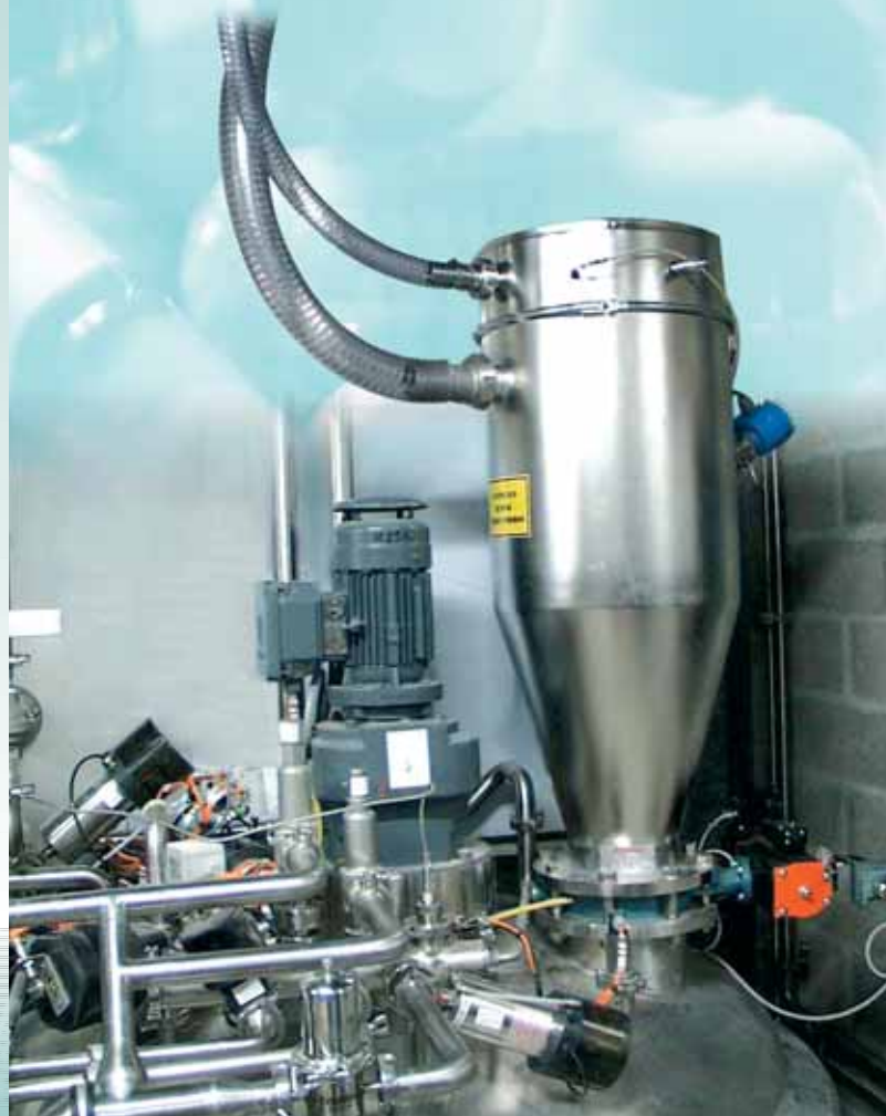
Easy dismantling by clamp collars
